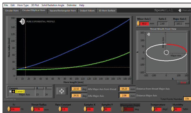
Figure 19: Elliptical mouth horns arrangement. MR = 2.4
